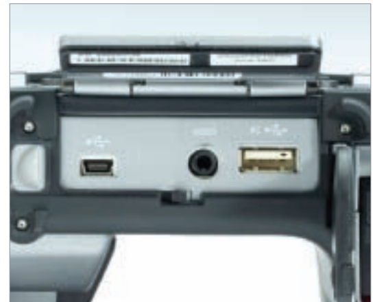
From Left to right: USB mini for PC image download, NTSC video, USB-A for memory stick image transfer
